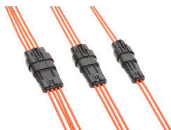
Squba 3.60mm-Pitch Sealed Connector Family, Fully Mated, 2 to 4 Circuits, with a Current of up to 14.0A
