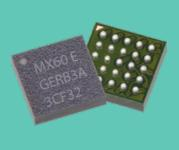
Contactless connectivity is paving the way for sleeker, more flexible and more durable technologies. Molex's **MX60 DisplayPort**, **MX60 Gigabit Ethernet** and **MX60 USB SuperSpeed Contactless Devices** offer high-speed, solid-state wireless connections with excellent reliability and robustness for harsh environments.
